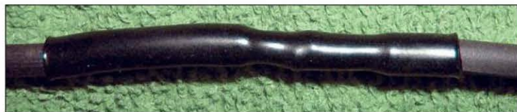
Figure 4 — Finish the splice with a piece of heat-shrink tubing for a neat and sturdy splice. [Frank Ingle, KG4CQK, photo]
