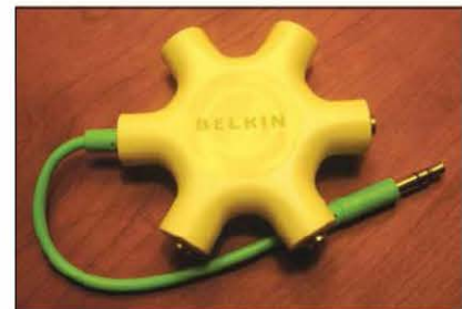
Figure 7 — The Belkin RockStar splitter is an inexpensive and neat method for connecting multiple accessories in your shack. [Bob Mayo, W2TAC, photo]
